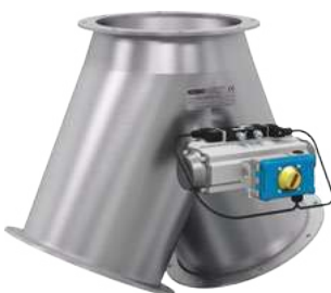
Example: Two-way valves with inner collar 50°, symmetrical, construction ND > 12" with welded-on flanges, pneumatically operated with a rotary actuator
